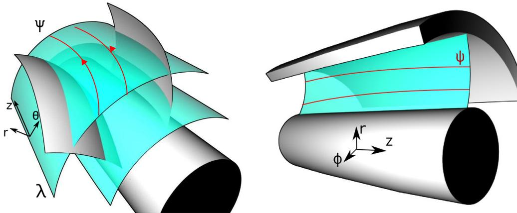
Figure 1: The 2D manifolds  $\lambda$  with streamlines  $\psi$  of two different flow problems: blade-to-blade and axisymmetric.
