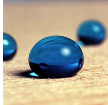
Water-repellent effect nanoparticle coating Courtesy of BASF
