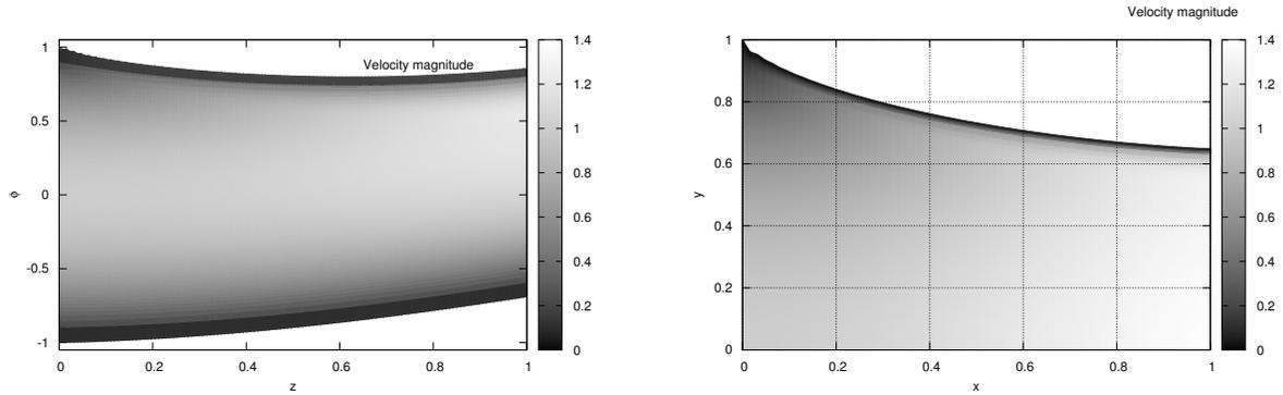
Figure 2: The nozzle and blade-to-blade channel design problem solutions.
