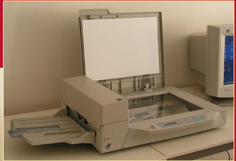
Document scanner FUJITSU M4097D: speed 60-90 pages in 1 min.
