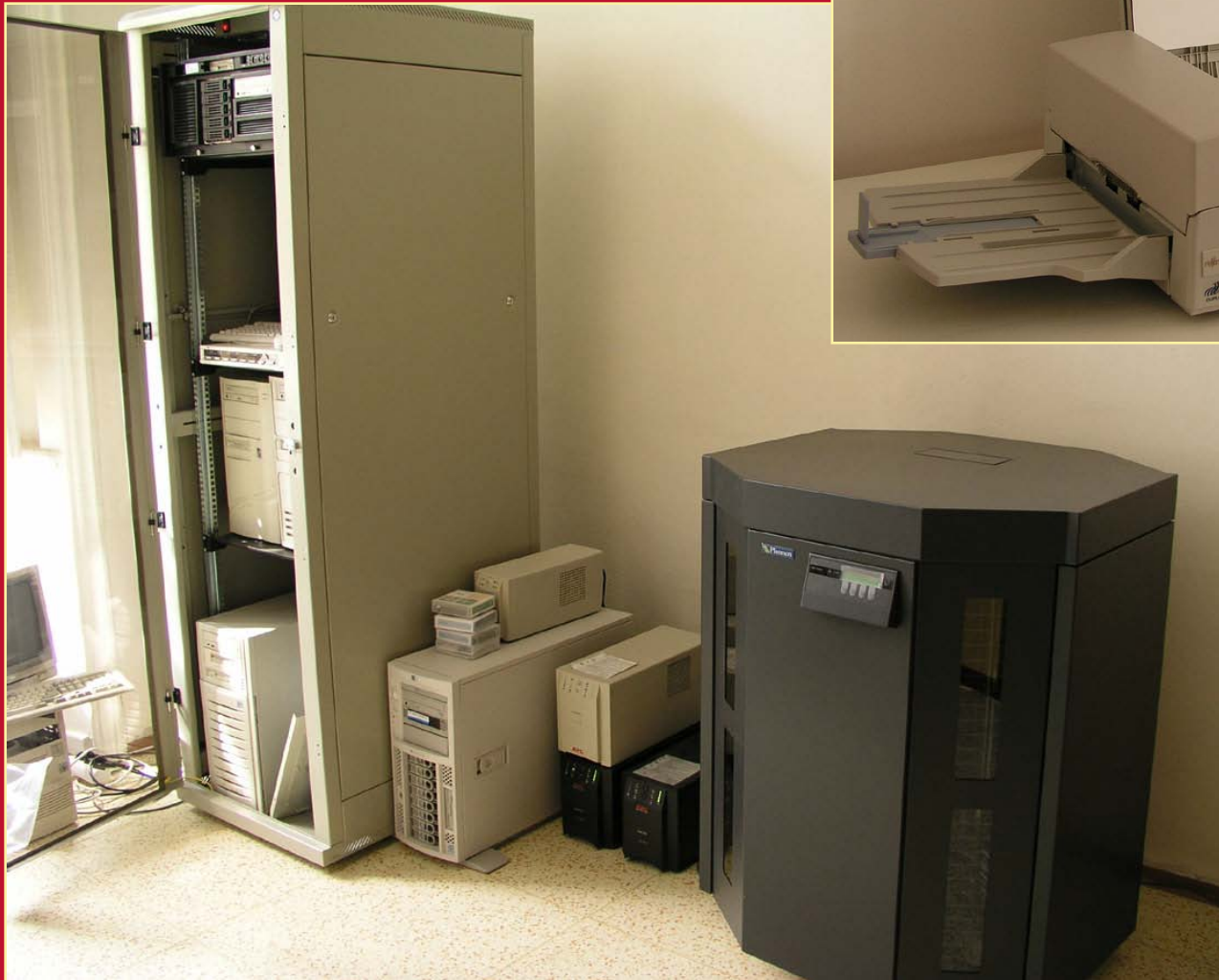
Jukebox PLASMON M104-910-X: 104 magneto-optical discs of 9.1 GBy each
