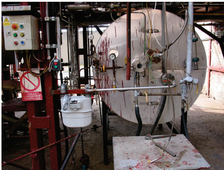
Afterburning furnace for incineration of the hydrogen
