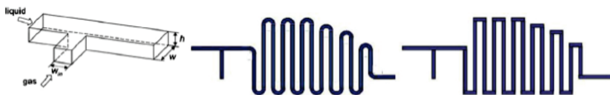
Schematic diagram of the T-junction microchannel (left) and the topology of the curved (center) and right-angled (right) meandering microchannels
