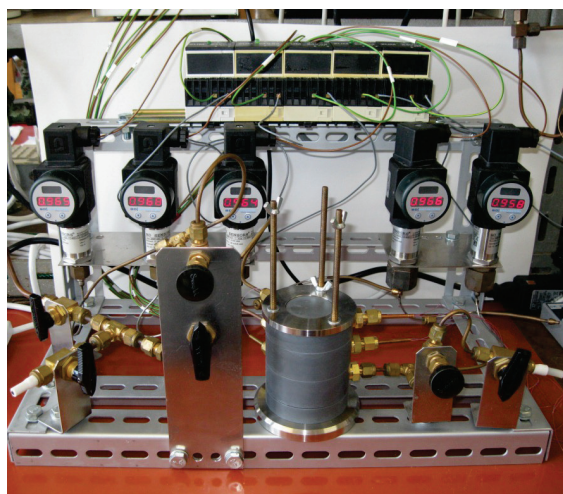
Apparatus for vapor permeation transport connected with condensation
