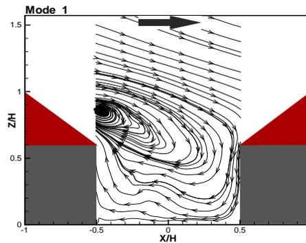
Figure 1: The most dominant POD mode derived from velocity data. Example of result from canyon with pitched roof.
