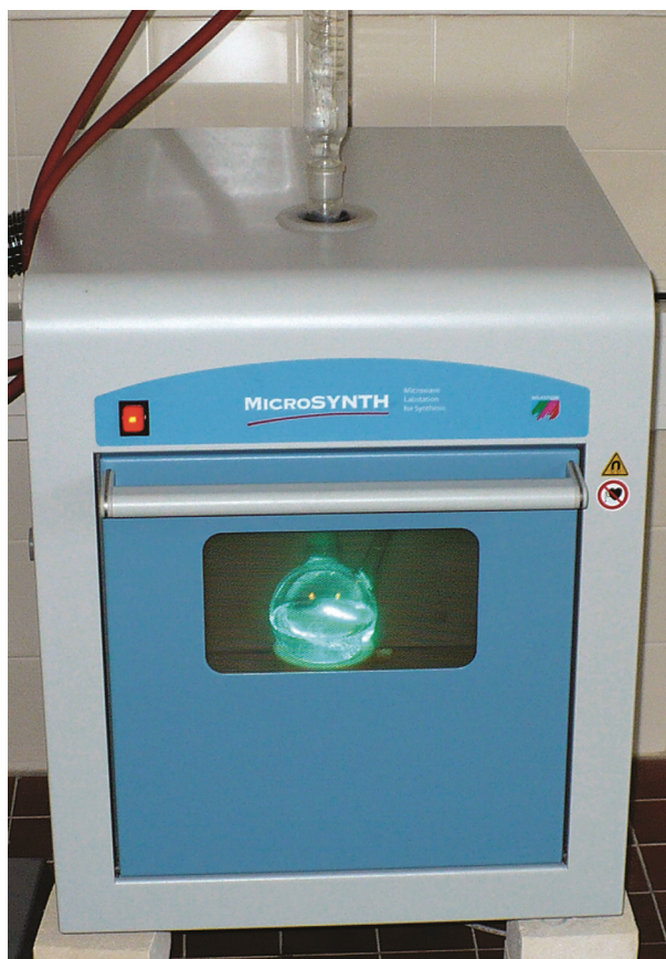
Figure 16. Microwave photocatalysis arrangement on Milestone's MicroSYNTH Labstation
