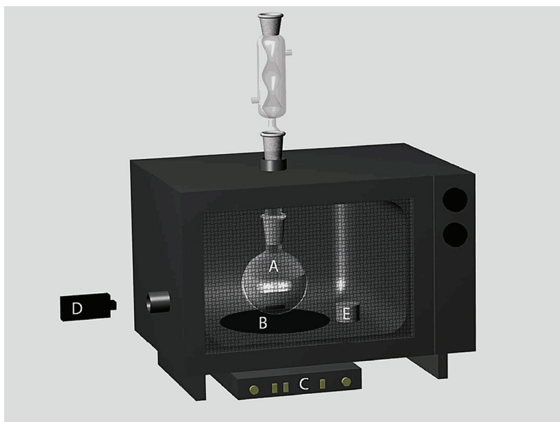
Figure 15. Modified MW oven for MW-assisted photochemical or photocatalytic experiments: (A) reaction mixture with EDL and a magnetic stir bar; (B) aluminum plate; (C) magnetic stirrer; (D) fiber optic spectral probe; (E) dummy load inside the oven cavity [132].
