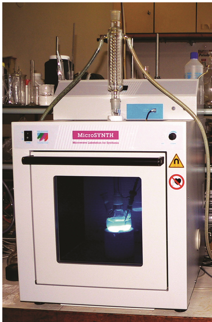
Figure 4. Testing the EDL performance in a Milestone's MicroSYNTH Labstation [25].
