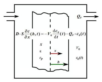
Fig. 1 Model of flow washing with retention
