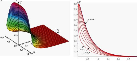
Fig. 2 Model of calcium hydroxide concentration field C in pelt in case of flow washing with retention
