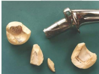
In vivo destroyed ceramic total hip joint endoprosthesis.
