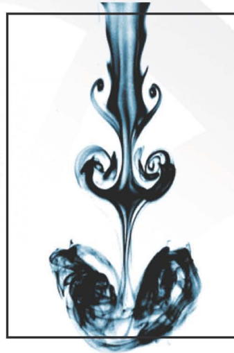
Coherent vortex lines in the shear layer and their breakdown, smoke visualization of submerged air jet.
