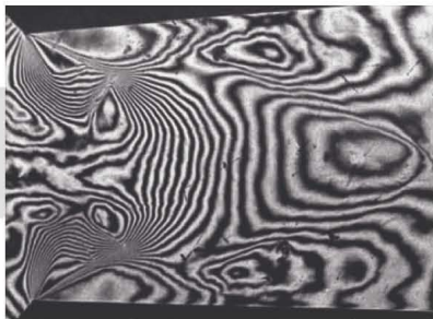
Interferogram of air flow in a control valve, the fringes correspond to regions of the same density.
