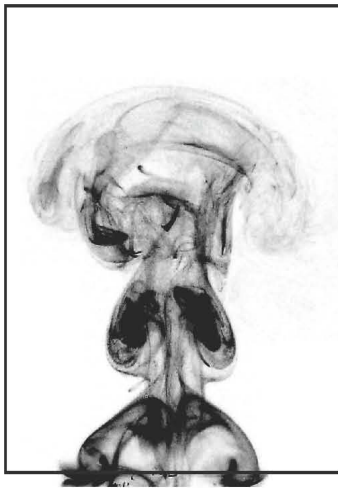
Smoke visualization of a synthetic jet.
