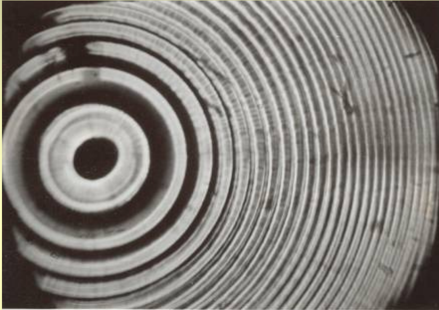
Microphoto of cross section of produced preform
