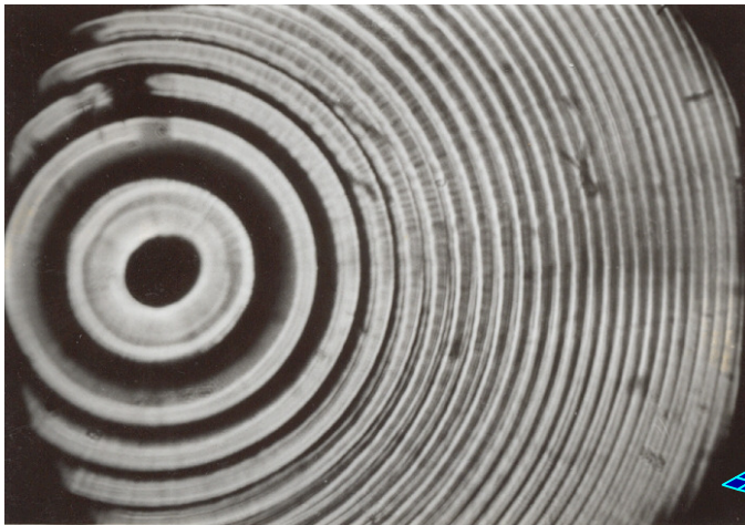
Microphoto of cross section of preform
