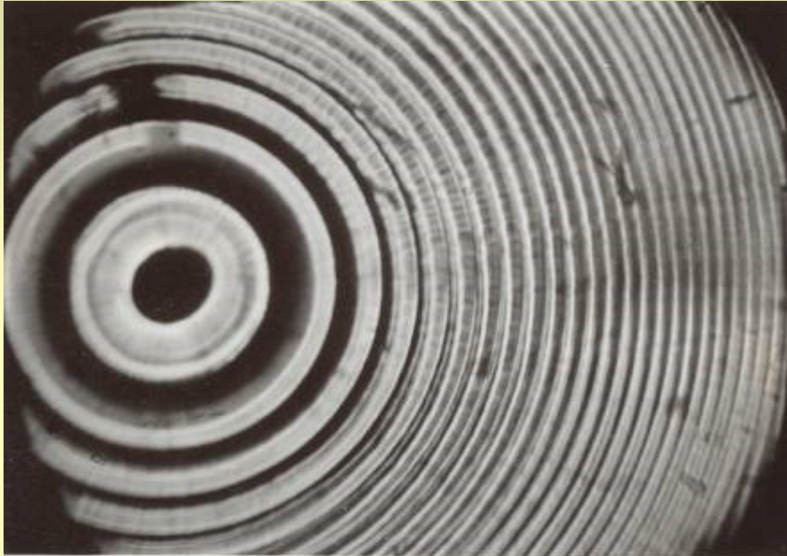
Microphoto of cross section of produced preform
