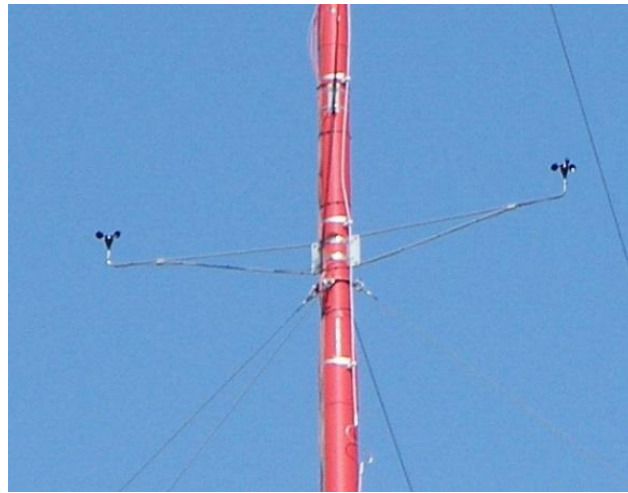
Figure 2 Wind mast measurement analyzed at Figure 3 . The anemometers are positioned 1.53 m (7.5 mast diameters) out of the wind mast of diameter 20.3 cm.
