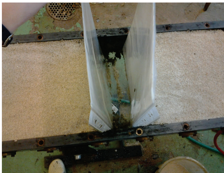
Detail of reactor filled up by sand with the prepared slot for sorbents
