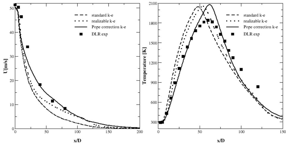
Figure 3. Axial velocity and temperature in the centerline.
