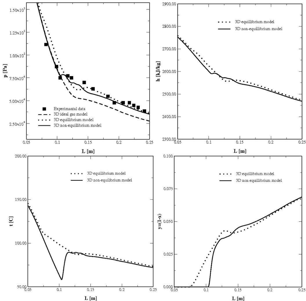
Fig.1. Pressure  $p$ , enthalpy  $h$ , temperature  $t$  and wetness fraction  $y=(1-x)$  changes in de Laval nozzle according to experimental data [1].
