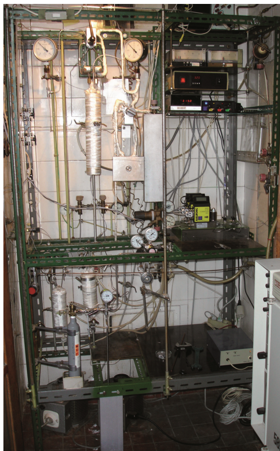
Pressure flow microreactor with fixed bed of catalyst for hydrodesulfurization
