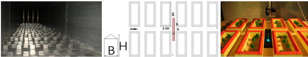
Figure 2: Left: roughness elements in testing section. Right: Scheme of building, model and photograph from experiment. Red lines denote the line source.
