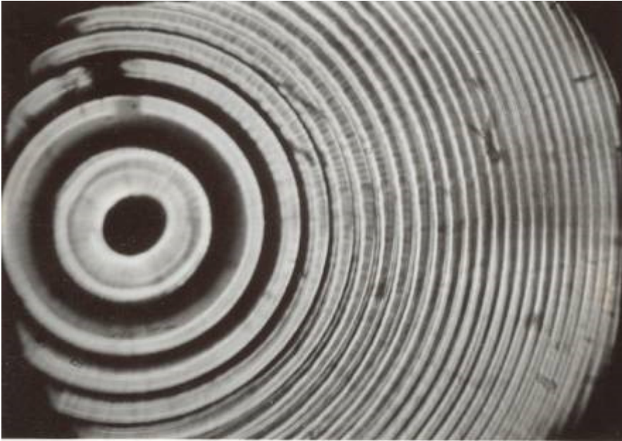
Microphoto of cross section of produced preform
