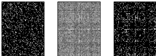
FIG. 1. An example of binary functional connectivity matrix (right) generated from random structural connectivity matrix (left) by thresholding the correlation matrix of AR-model generated time series (center, light shades of gray indicate higher correlation values). Network with N = 100 nodes shown. Note that the functional connectivity matrix shows a specific structure although the entries of the generating structural connectivity matrix were chosen randomly. See text for further details.
