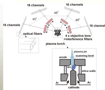
**Arc length 5 mm, nozzle diameter 6 mm, arc current 200 A, argon flow rate 1 g/s, plasma jet radiation scanned 5 mm above nozzle, interference filters with the maximal transmittance at 650 nm and spectral width 80 nm, sample rate 468 kHz/channel and record lengths 1 Msample/channel.**
