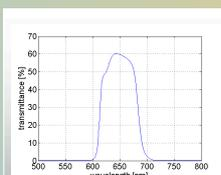
**Spectral characteristics of interference filter.**
