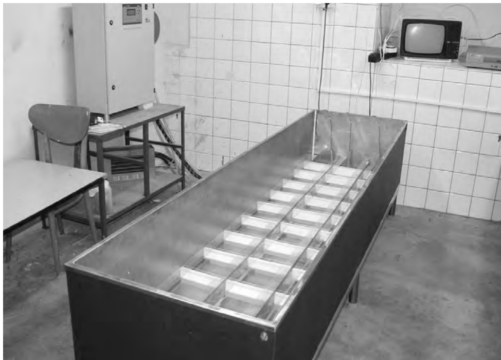
Horizontal thermal gradient (5 - 32.5°C) for measuring temperature preferences in aquatic animals.
