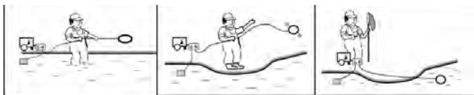
PAS electrofishing techniques: direct, thrown anode and remote electrofishing.
