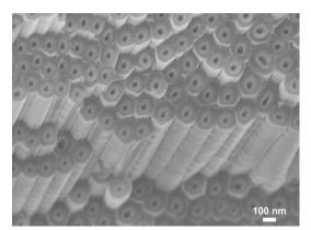
SEM image of Al<sub>2</sub>O<sub>3</sub> coated self-organized TiO<sub>2</sub> nanotubes by Atomic Layer Deposition
