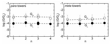
Figure 3. Length dependence of the average molecular conductance values.
