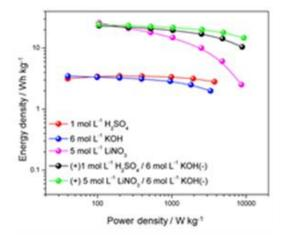
**Fig. 2** Ragone plot for the various hybrid capacitor systems
