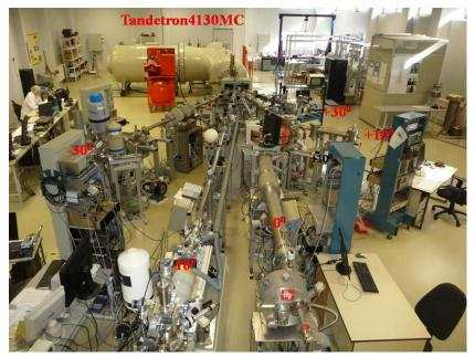
• Low energy ion beams, produced by small accelerators, penetrate matter and interact with atoms to produce X-rays,  $\gamma$ -rays and other particles which provide information about the structure and composition of the object.
