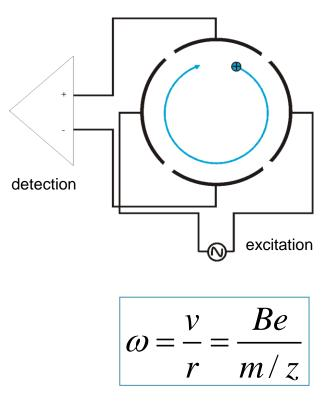
Detector electrodes measure the electrical signal of ions which pass near them over time, producing a periodic signal
