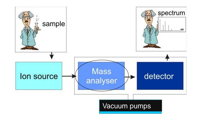
Mass analysers - separate the ions according to their mass-to-charge ratio
