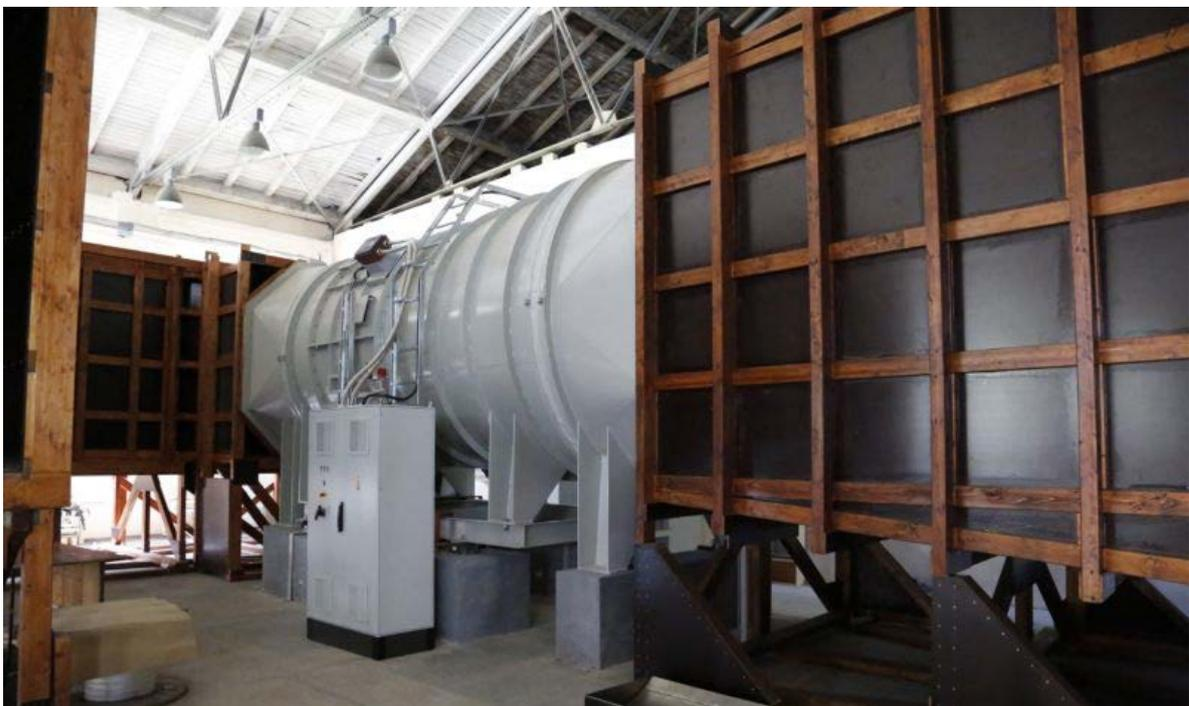
Fig . 2 Overview of the WT power unit and its control system.
