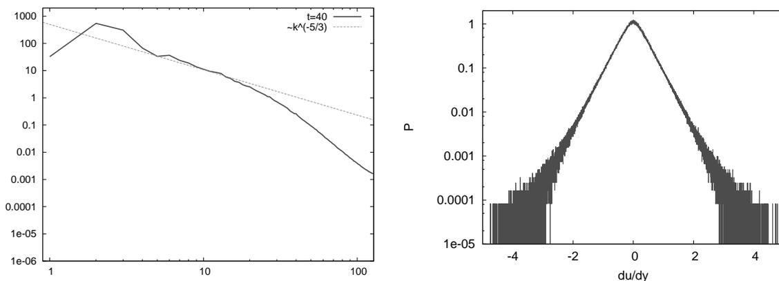
Figure 1: a) The energy spectrum at  $t = 40$ , b) A PDF of  $\frac{\partial u}{\partial y}$ .
