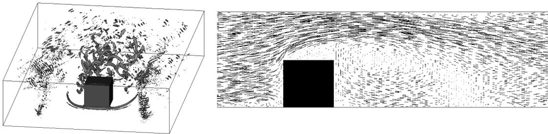
Figure 2: a) A snapshot of visualized vortices behind the cube, b) An averaged flow field in a  $xz$  plane of symmetry.
