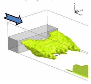
The high positive vertical velocity component region in trident shape was studied in details. As the maximal value of the vertical velocity is about 0.6 m/s. The structure originates in corners on the top of the step forming two elongated structures, the third elongated structure arises in the middle of the channel.
