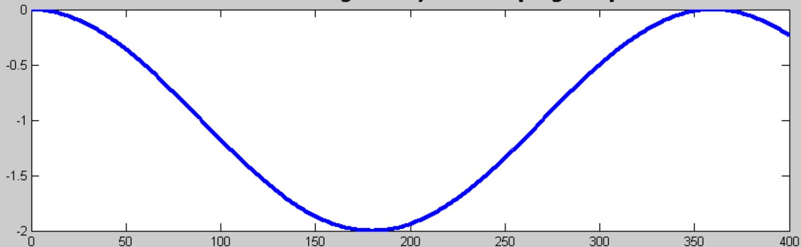
stress11 [ $\text{N}/\text{m}^2$ ] vs. rigid body rotation [degrees]
