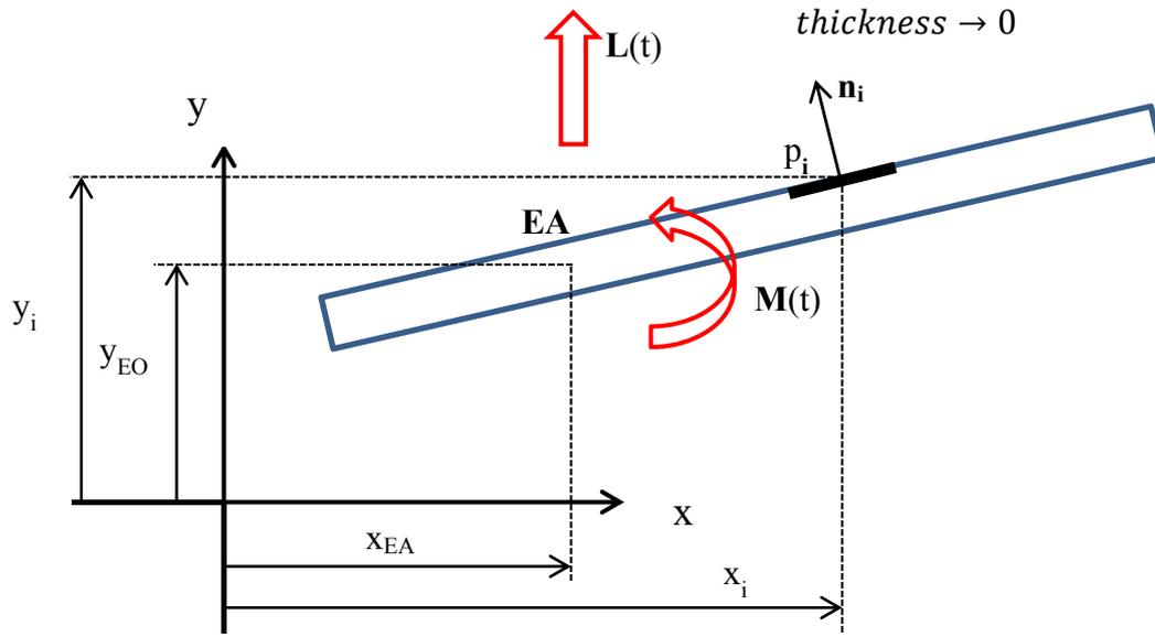
Figure 3: Scheme for calculation of the forces acting on the airfoil.
