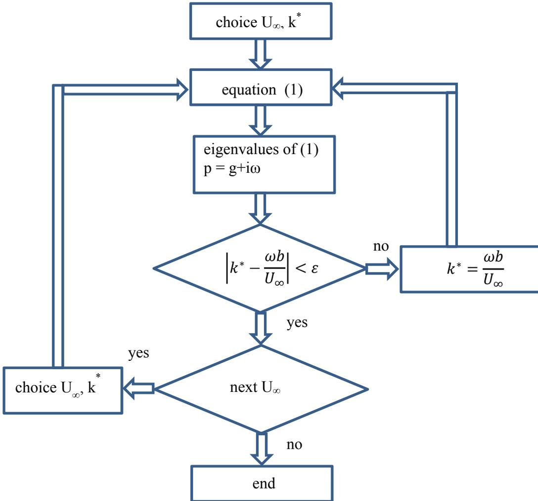
Figure 2: The p-k algorithm is based on iterative procedure
