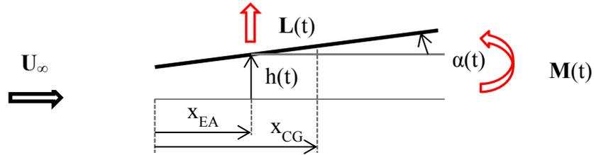
Figure 1: Scheme of the airfoil with center of gravity (CG) and elastic axis (EA) vibrating with two degrees of freedom.
