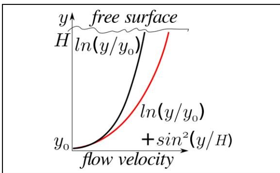
Fig. 6 The velocity profiles: standard averaged turbulent profile (the log-law) and profile with influence of the flow depth and wavy surface.
