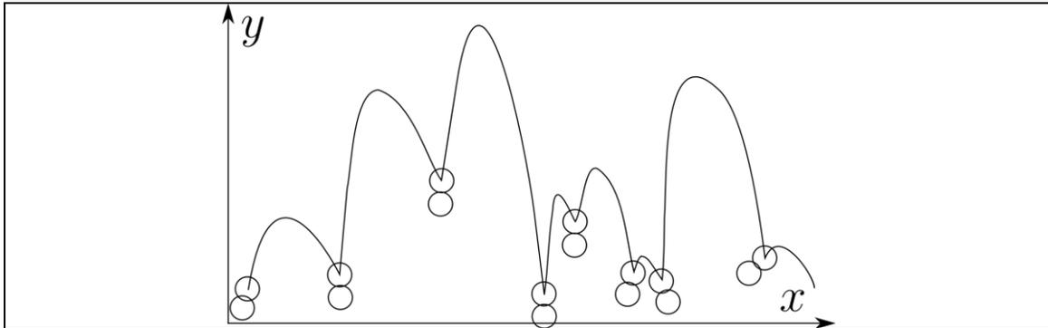
Fig. 5 A hypothetical trajectory of the saltating particle after its collisions with other conveyed particles and bed particles.
