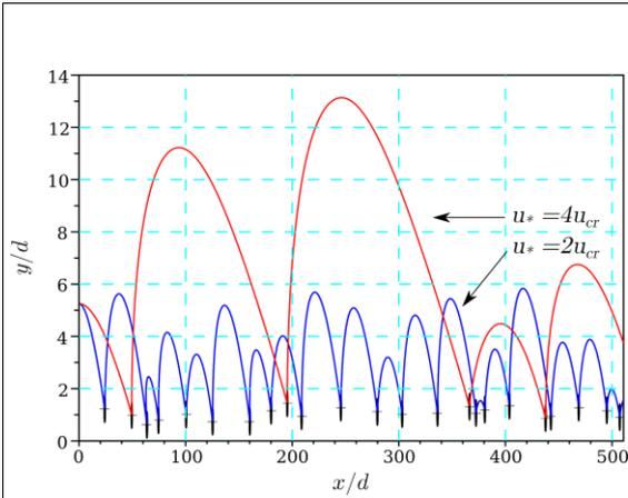
Fig. 1 Saltation of one particle with various flow velocities: effect of shear velocity on trajectory.
