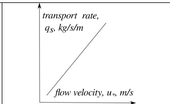
Fig. 7. Tentative dependence of bed load transport rate,  $q_s$ , on flow velocity,  $u_*$ .
