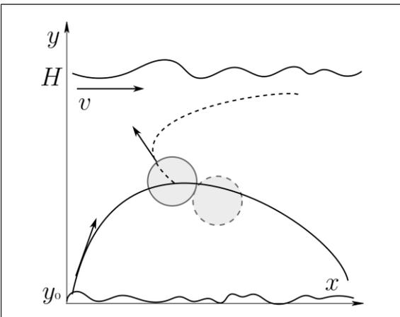
Fig. 3 The sketch of particle-particle collision. Dashed line – new trajectory of the saltating particle after collision with hypothetical particle.
