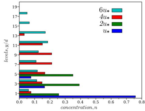
Fig. 2 Normalized concentration of the saltating particles in the separate layers [0-2; 2-4; ...]  $d$  for various flow velocities,  $u^*$ . Depth of the flow is  $H = 20 d$ .
