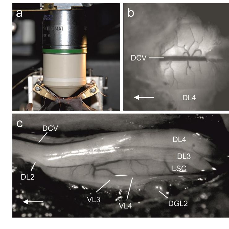
**Figure 3** Mounted vertebral column with spinal cord ready for microscopy. (a) Vertebral column fixed by clamps; objective lens in position. (b) Dorsal aspect of the spinal cord; view through the cleft between lumbar spines 1 and 2; dura intact. (c) Lateral aspect of the spinal cord; spinal arcs L1 to L3 dorsally and on the left side completely removed; dorsal roots L3 and L4 shifted dorsally. Arrows show rostrally. DCV: dorsal central vein, DGL: lumbar dorsal
