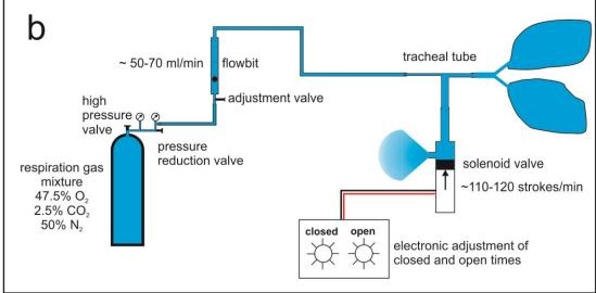
**Figure 2** Infusion anesthesia and artificial ventilation. (a) Ventral aspect of the mouse neck, with central vein catheter and tracheal tube. (b) Diagram of respiration gas flow during artificial respiration.
