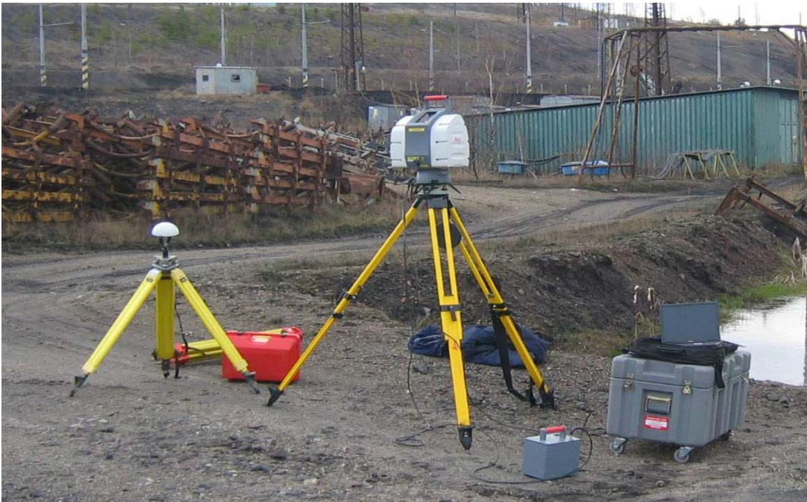
The High-Definition Surveying (HDS) scanner for a versatile and very accurate 3D laser scanning, which uses a high-speed laser and a built-in digital camera to rapidly photograph and measure a scene
