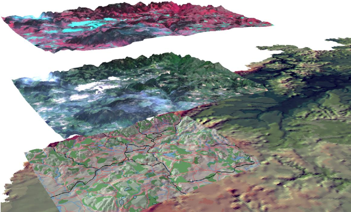
The satellite images of the surface coal mine from Landsat 7 ETM+ draped on the DTM based on contour lines (a pseudo colour composite with bands 4-3-2 above a true colour composite with bands 3-2-1, thematic map layers in the bottom part)
