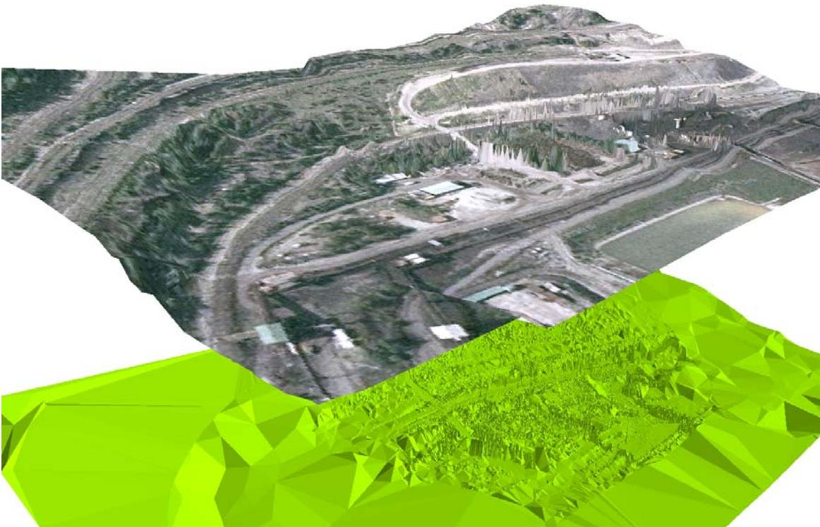
The aerial image of the slope located in the coal mine draped on the DTM based on GPS data, geodetic survey and laser scanning (a true colour composite of the aerial image above the DTM assembled by the TIN data)
