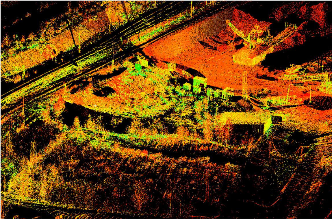
The clouds of the 3D points captured by the surface laser scanner from a few positions and merged by software tools for creation of the DTM
