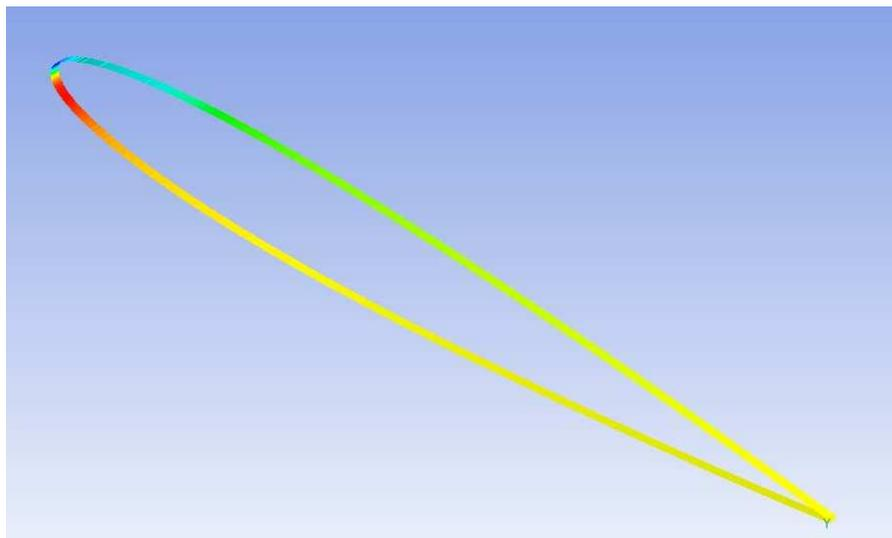
Fig. 11. Wall pressure distribution along the airfoil surface.
