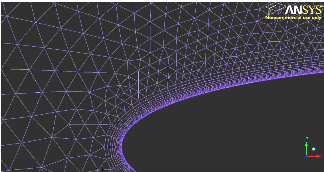
Fig. 7. Grid details near the airfoil surface.
