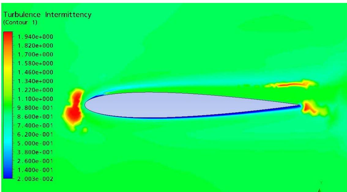
Fig. 9. Turbulence intermittency near the airfoil.
