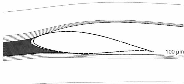
Fig. 1. Illustration of the water droplets trajectories. Airfoil NACA 633 418, water content  $1 \text{ g}\cdot\text{m}^{-3}$ , velocity  $50 \text{ m}\cdot\text{s}^{-1}$ , angle of attack  $5^\circ$ .
