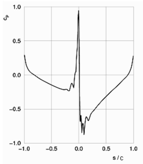
Fig. 2. Example of pressure coefficient  $c_p$  on dimensionless airfoil surface length  $s/c$ . Clean airfoil NACA 0012, chord  $c = 0.1$  m, velocity  $20 \text{ m}\cdot\text{s}^{-1}$ , angle of attack  $2^\circ$ .
