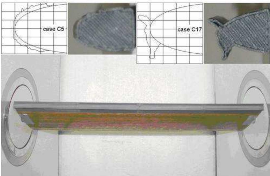
Fig. 4. Model of iced NACA0012 airfoil in the wind tunnel test section.
