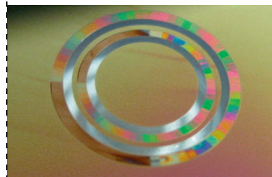
Combined phase / amplitude photo mask for vortex beam generation
