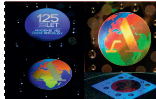
Examples of optically variable devices originated on variable-shape EBPG BS600 in TZ mode (above) and Gaussian-type EBPG Vistec (below)
