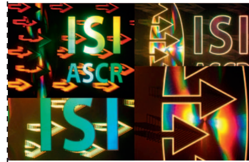
Examples of optically variable devices originated on variable-shape EBPG BS600 in TZ mode (above) and Gaussian-type EBPG Vistec (below)
