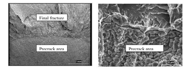
Fig. 5. Crack tip of weld metals, no crack growth covered with oxide initiation was indicated.
