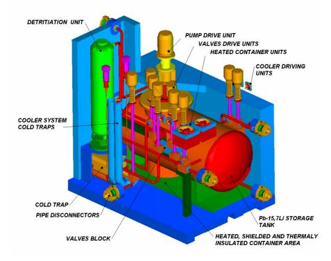
Fig. 2. View of the Pb-17Li auxiliary system for ITER HCLL TBM
