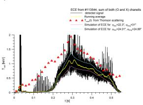
**Fig. 2.** The time development of EBW signal (sum of O and X channels) detected by the NSTX antenna operating at 16.5 GHz. #113544.
