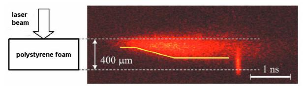
**Fig. 1** *X-ray streak record of the thermal wave penetration into the polystyrene foam layer 400 μm thick (foam density 9mg/cm<sup>3</sup>, pore diameter 50–70 μm).*
