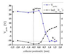
Fig. 2. Dependence of the BPP signals on the collector position. The probe potential  $(V_{probe})$  and ln(R).
