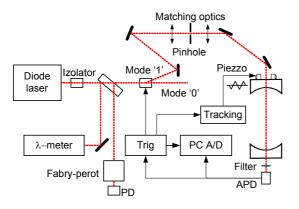
Fig. 1. The experimental set-up.
