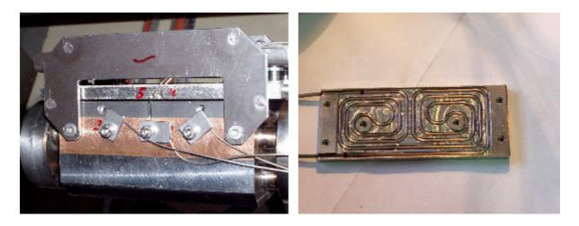
Fig. 15. Instrumented Primary First Wall mock-up Fig. 16. Nickel heating panel with Thermocoax specimen prepared for out-of-pile test heating wire
