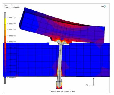
**Fig. 17.** Von Mises stress distribution in the PFW panel, supporting plate and attachment stud under prescribed poloidal moment. The deformation of the test objects (magnification factor 200)
