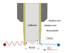
**Fig. 1.** *Schematic picture of the ball-pen probe.*
