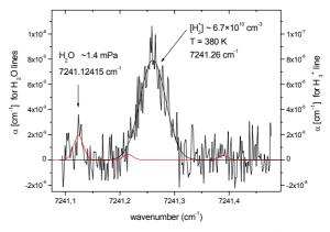
**Fig. 2.** The absorption spectra of  $H_3^+(v=0)$  obtained in a continuous microwave discharge in He with admixture of hydrogen.
