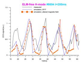
**Fig. 1.** Comparison of the detected ECE signal and two simulations: EFIT magnetic equilibrium and the equilibrium with a bump in the magnetic field profile at the transport barrier.
