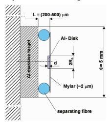
Fig. 3 The target holder used in the double-target experiments.
