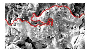
**Fig. 4.** The detail of the irradiated tungsten surface (SEM image, magnification 500x). The smooth metallic surface of the bright "branch" (without oxides) is on the top.
