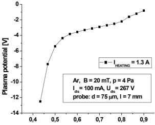
Fig. 2. Radial profile of plasma potential obtained by emissive probe in magnetron.
