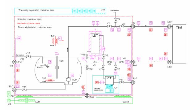
Fig. 1. Schematic layout of the Pb-17Li auxiliary system for the HCLL TBM
