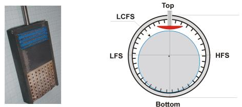
**Fig. 1** *Left - Picture* of the 2D matrix of 64 Langmuir probes. *Right - Schematic picture of the poloidal cross-section of the CASTOR tokamak showing the respective position of the biasing electrode, the plasma column and the poloidal limiter.*
