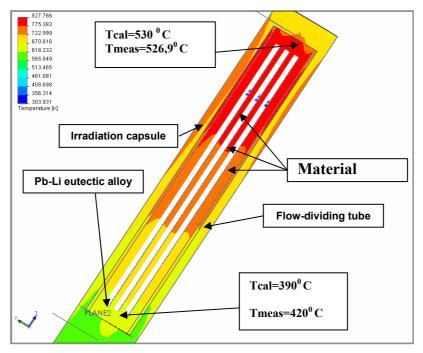
**Fig. 11.** Comparison of calculated and measured temperatures in the Pb-17Li in-pile rig at reactor power 9 MW
