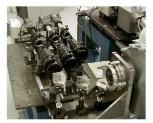
**Fig. 2** View of the detection part of the 3-frame interferometer.
