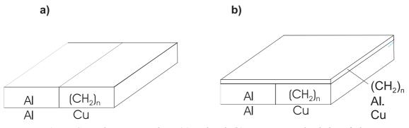
Fig. 5 Cascade targets without (a) and with (b) a covering polyethylene foil.
