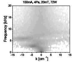
**Fig. 1.** Frequency wave number histogram of the fluctuations observed in DC discharge in cylindrical magnetron. From [2].
