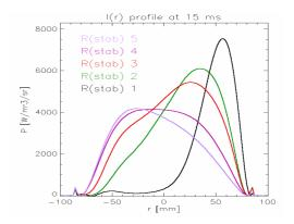
**Fig. 4.** A bolometrically measured radial distribution of the radiated power for 5 different settings of the horizontal stabilization system of the CASTOR tokamak at 15 ms.
