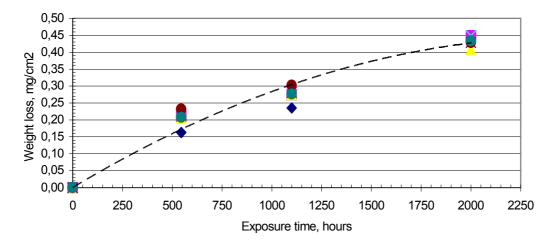
Fig. 7. EUROFER tube specimens weight loss under PWR conditions
