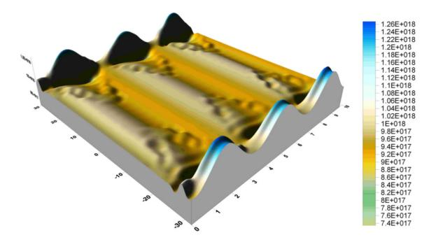
**Fig. 1.** Dependence of the plasma density in front of three wave-guide rows of a LH grill launcher, the parameters correspond to the Tore Supra C3 launcher.
