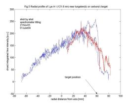
Fig. 1. Radial profile of H I Ly $\alpha$  121.6 nm near tungsten (blue) and carbon (red) targets.
