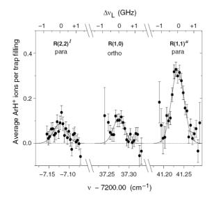
**Fig. 3.** Measured absorption profiles for the three observed transitions in the  $(0,3^1) \leftarrow (0,0^0)$  vibrational overtone band. The employed chemical probing technique yields an  $ArH^+$  ion per absorbed infrared photon. The signal is derived by averaging over 500 trap fillings, interleaved by 500 background measurements. The absolute accuracy of the frequency scale is  $\pm 0.017$  cm<sup>-1</sup>.
