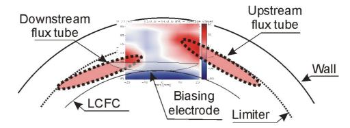
**Fig. 3.** Poloidal projection of the biased flux tube as measured by the 2D matrix of Langmuir probes. The lengths of the downstream and upstream tubes are ~30 cm and 220 cm, respectively.
