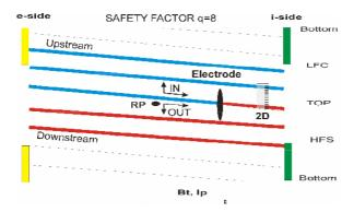
Fig. 2. Biased flux tube originating at the electrode is shown schematically on an unfolded magnetic surface in the SOL for  $q_{edge} \sim 8$ . The toroidal location of the rake probe and of the 2D matrix is marked.
