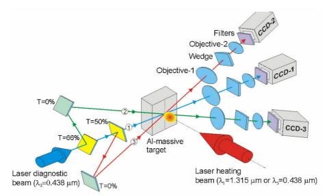
Fig. 1 Simplified scheme of the 3-frame interferometric system exploited at PALS.
