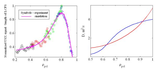
**Fig. 1.** *The experimental profile measured by USX is plotted together with the simulated one. The same result is obtained by both profiles of diffusion coefficients on the right.*
