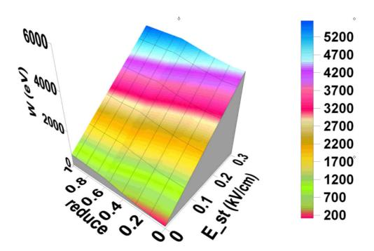
**Fig. 2.** The maximum accelerated electron energy W (eV) as a function of the parameter "reduce" and as a function of the varying random field amplitudes  $E_{st}$ .
