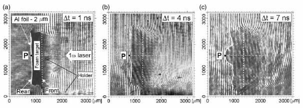
**Fig.** 2 Sequence of interferograms/shadowgrams showing the acceleration of Al foil attached to the rear side of the 400-μm thick polystyrene foam target.
