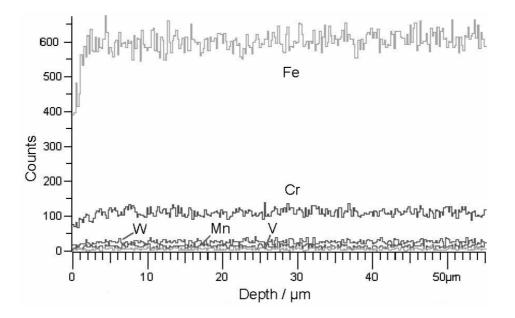
Fig. 9. EDX line scan of specimen cross-section after 2000 hrs exposure in Pb-17Li at 500°C.
