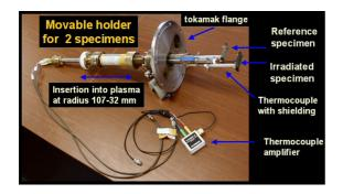
**Fig. 3.** The movable holder for the insertion of two plasma-sprayed tungsten specimens into a tokamak chamber.
