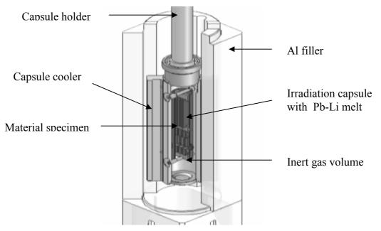
Fig. 10. Design of Pb-17Li in-pile rig.
