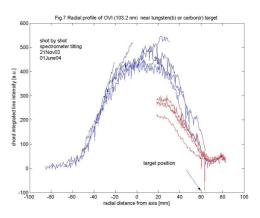
**Fig. 2.** Radial profile of O VI 103.2 nm near tungsten (blue) and carbon (red) targets.
