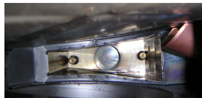
Fig. 2 Detail of shaped antenna mouth place in the narrow tokamak port
