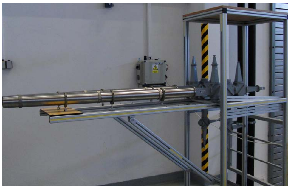
Fig. 2. Picture of the built-up BCA on the support structure
