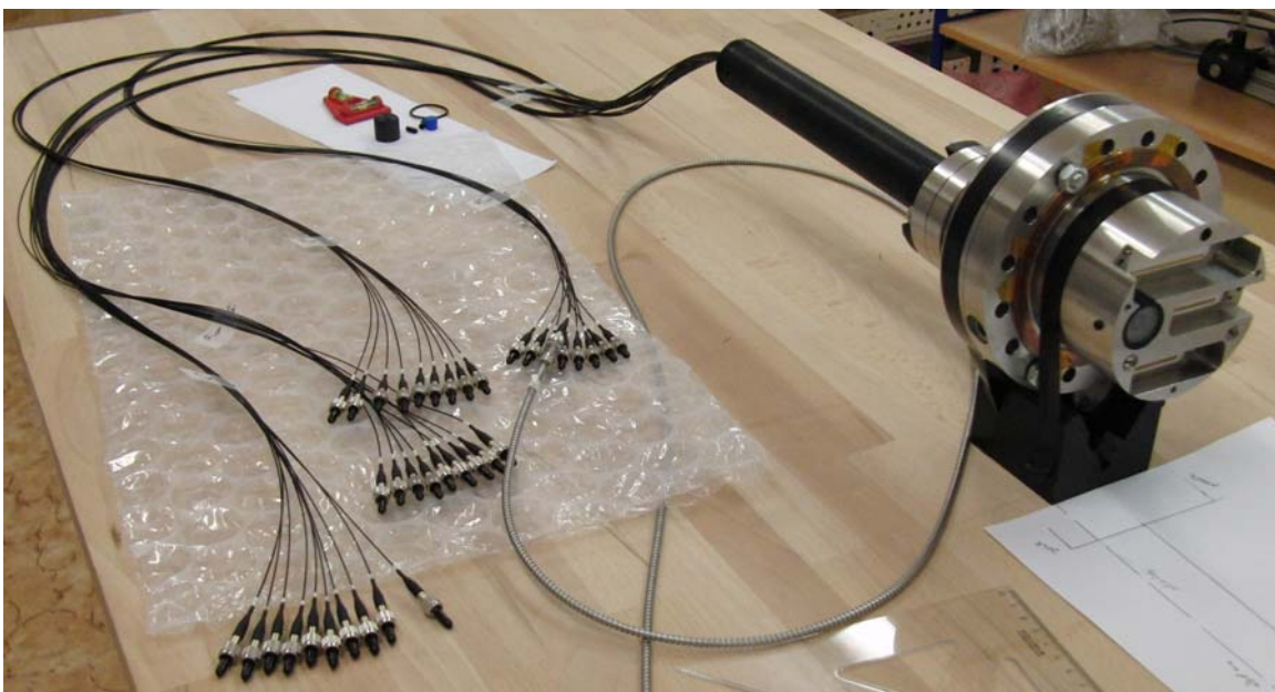
Fig.1: Laboratory tests on the completed integrated spectroscopic port plug. The objective consisting of the vacuum and atmospheric parts is connected to the fiber optics.
