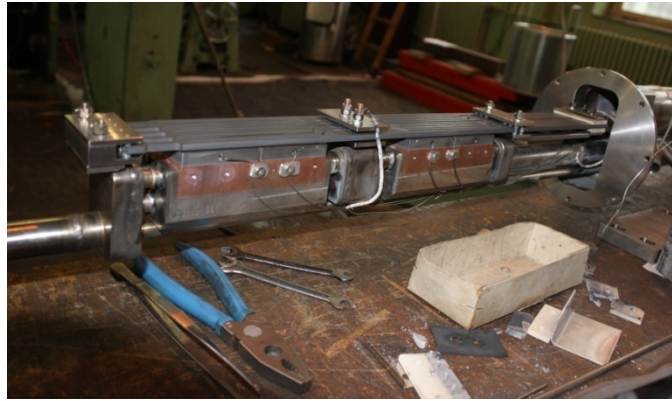
Fig 3: Final design modifications on TW3 irradiation rig before last out-of-pile test; same design will be used for in-pile testing.
