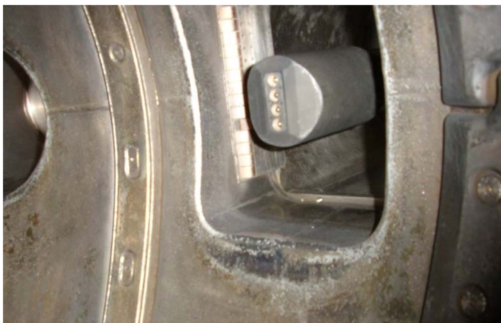
Fig. 1: Photograph of horizontal probe head inside the COMPASS vacuum chamber.
