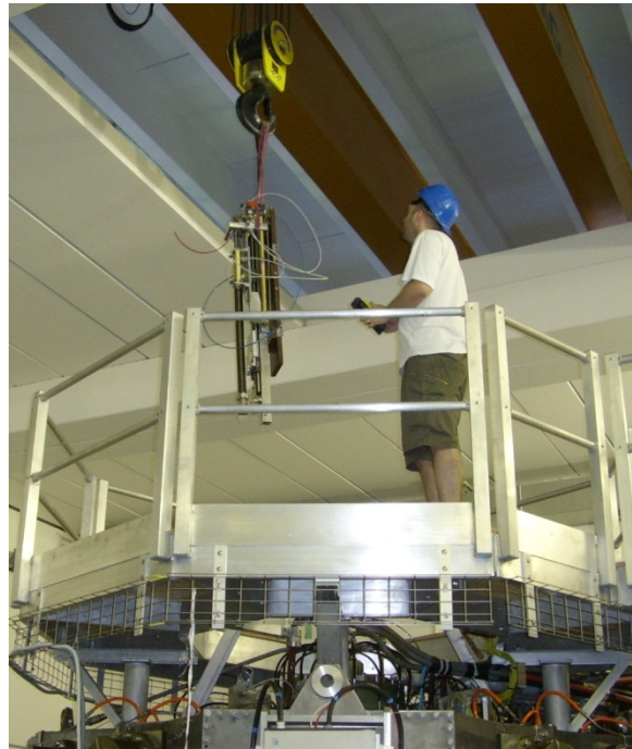
Fig. 2: The vertical probe during installation on the top port of COMPASS.
