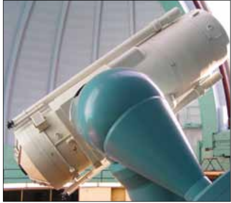
The Perek 2-m telescope is the primary instrument in the Ondřejov observatory.
