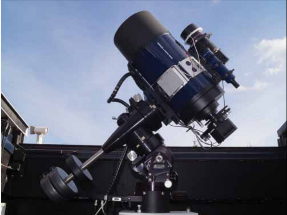
The 0,25-m BART telescope of the GLORIA project located in one of the domes of the Institute.
