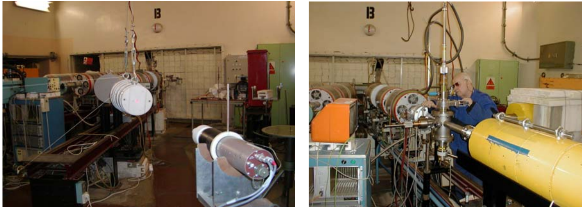
Fig. 2. The experimental arrangement of the neutron transport- (left side) and cross-section measurements (right-side) employing the NG1 target station.
