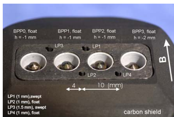
Fig.1. Picture of the quadruple ball-pen probe used in AUG during the campaign in 2009. The probe head has four BPPs with conical tips retracted into the boron nitride screen. In addition, there are four graphite Langmuir probes.
