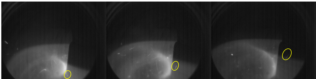
Fig. 3. Formation of circular plasma at 6 th ms in the discharge #323 and a dust particle tracking demonstrated on three consecutive camera frames of 800x600 pixels spaced in time by 1.475 ms.
