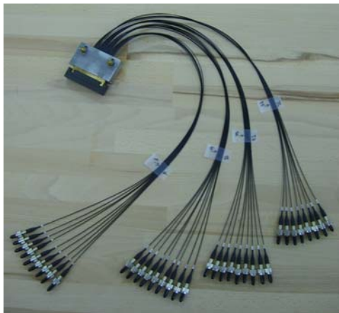
Fig. 1. "Detector side" endpiece. It consists of the 35-channel connector equipped with a protection shielding and 50 cm optical cables with SMA connectors at the ends.
