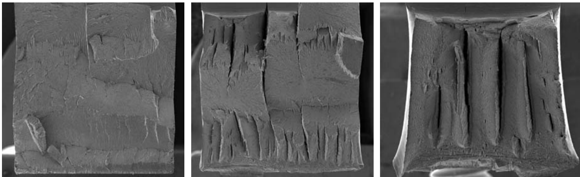
Fig. 3. Fracture surfaces of 18Cr-1W-0.19Ti-0.3Y 2 O 3 steel fractured near LSE, T_{DBTT} and USE, overviews.
