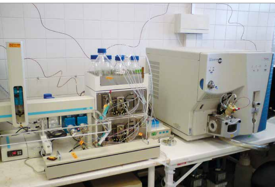
Figure 1: LC-MS system TSQ Quantum Ultra AM with Rheos 2200 chromatograph and CTC HTS autosampler
