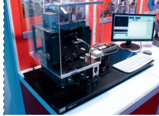
Nanocomparator for interferometric calibration of displacement sensors for the automotive industry
