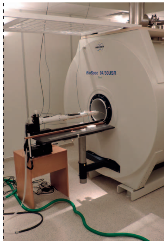
Preclinical 9.4T MR scanner equipped for mouse, rat and rabbit imaging
