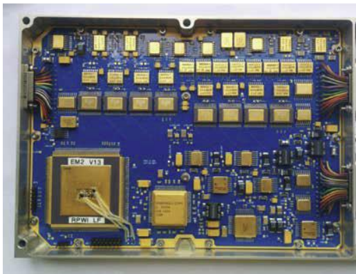
Figure: Left: Engineering model of the LF module for JUICE RPW1 which will analyze measurements of the electric and magnetic field. Right: Electronics board of the power supply for the RPW1 experiment on JUICE space probe during one of the ground tests. Depicted is engineering model 2B.
