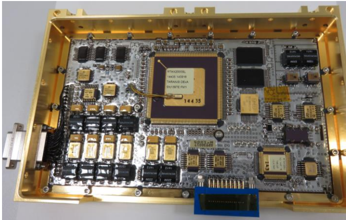
Figure: Flight model of the TARANIS IDEE DZA data processing unit (FMP CU delivered two flight models). The DZA and DNA units are part of the MEXIC-1 electronic box.
