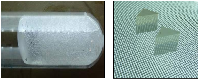
Figures: Growing and annealed Calomel crystal and polished Calomel optical components.
