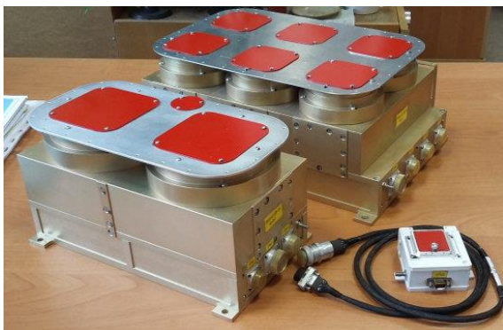
Figure: Mechanical prototypes of the BMSW-LG detector blocks (a heritage of the Spektr-R BMSW instrument working in orbit since 2011).
