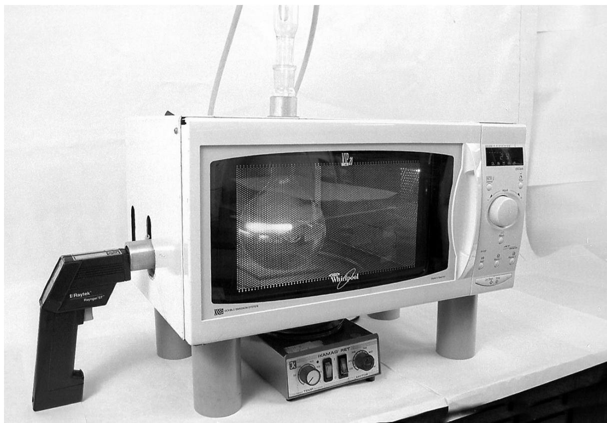
**Fig. 14.6** Photochemistry in a microwave oven (EDL floats on the liquid surface).
