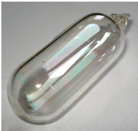
Fig. 1. The titania thin film coated EDL.
