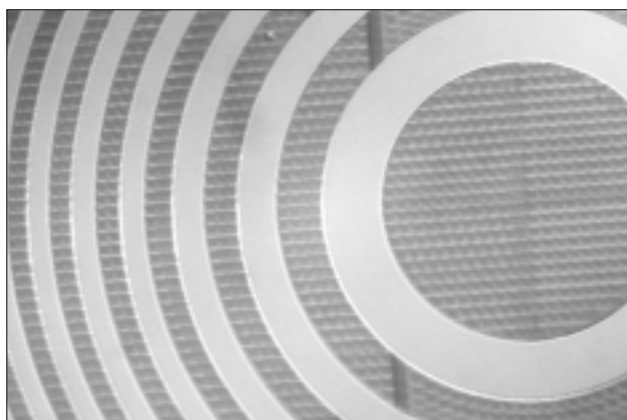
Fig.1. The central part of diffractive lens microstructure in a negative electron resist (magnification 500)
