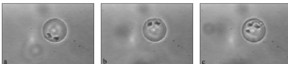
Fig.2. Spontaneous rotation of a 15 μm sphere irradiated by a continually working laser. The holes on the sphere top were made using a pulsed laser. They cause the photons to leave the sphere in an asymmetric way, which leads to the sphere rotation (note the change in the position in figures a and b ). In figure c , another hole was made.
