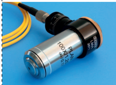
An example of compact optical tweezers developed in collaboration with Meopta company
